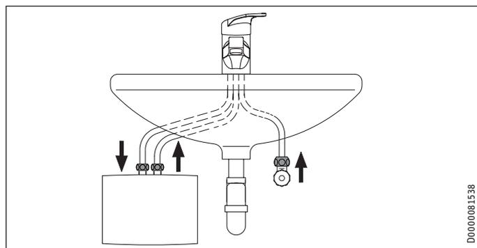
Connect the short connection hose marked blue to the angle valve of the cold water supply line.
