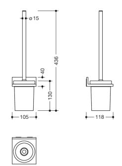
Abmessungen in mm
