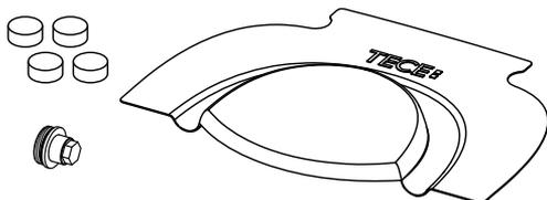
To use the descaling set, you will need a 2.5 mm Allen key, a socket spanner with a 17 mm nut, needle-nose pliers and a thermometer (optional). For your own safety, we recommend that you wear gloves and safety glasses.
