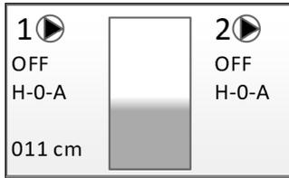
The standard display shows the operating mode of the control unit, the switching status, the motor current and the level.
