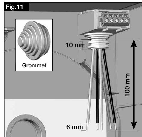
The connection cable must be stored so that water cannot penetrate along the cable in case of water exposure. The cable must not pass over sharp edges!
